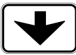
R7-5 B size 450 x 300 C size 600 x 400 D size 900 x 600 E size 1200 x 800
