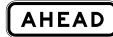
R7-2 B size 450 x 150 C size 600 x 200 D size 900 x 300 E size 1200 x 400
