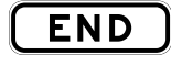
R7-4 A size 300 x 100 B size 450 x 150 C size 600 x 200 D size 900 x 300 E size 1200 x 400
