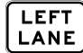
R7-3(L) B size 450 x 300 C size 600 x 400 D size 900 x 600 E size 1200 x 800
