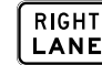
R7-3(R) B size 450 x 300 C size 600 x 400 D size 900 x 600 E size 1200 x 800
